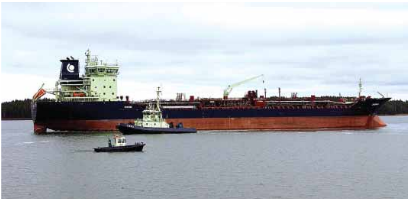
Purha is a double-hull tanker, constructed for carrying chemical and oil products in the Baltic Sea and North Sea from Fortum's refineries in Porvoo and Naantali.
