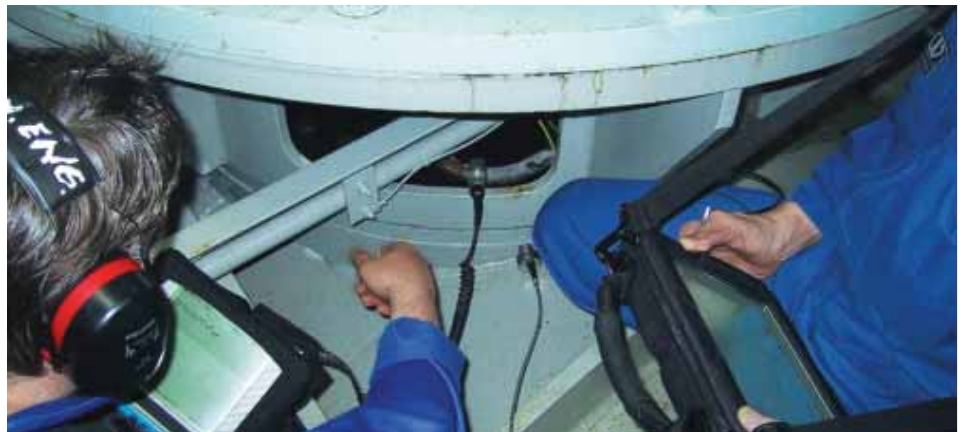
Vibration monitoring of a thruster by the crew and DNV during an implementation survey.
