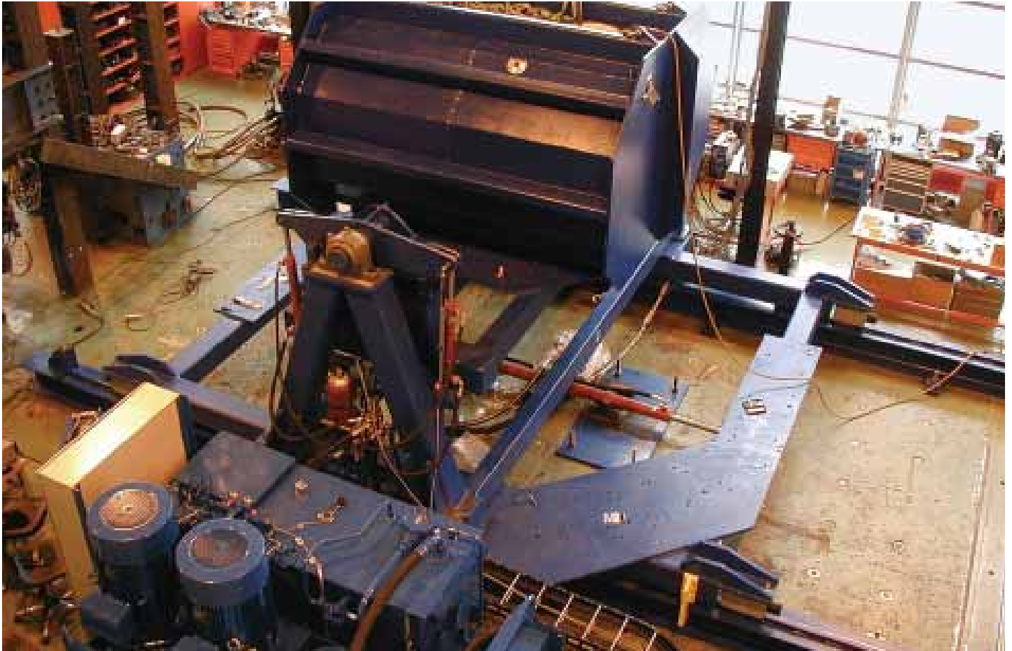
The sloshing test platform developed by DNV for its current R&D programme.
