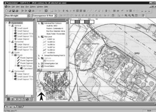
Figure 1 – Typical Individual Risk Contours displayed using SAFETI
